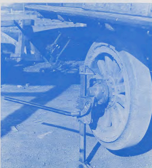
A lifting jack, made in our plant, in action.
